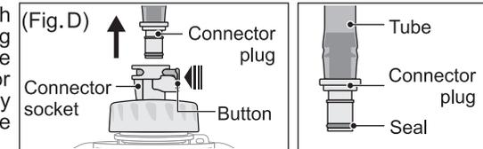
\*When detaching the tube, make sure the seal is still attached to the tube. The seal has a definite lifespan. When the tube is attached correctly but water is leaking, it is time to replace the seal.
